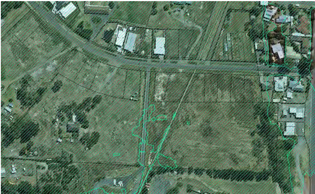
Figure 9 Coastal Inundation Hazard Area Overlay in green hatching (High Medium and Low) (source: thelist.tas.gov.au)
