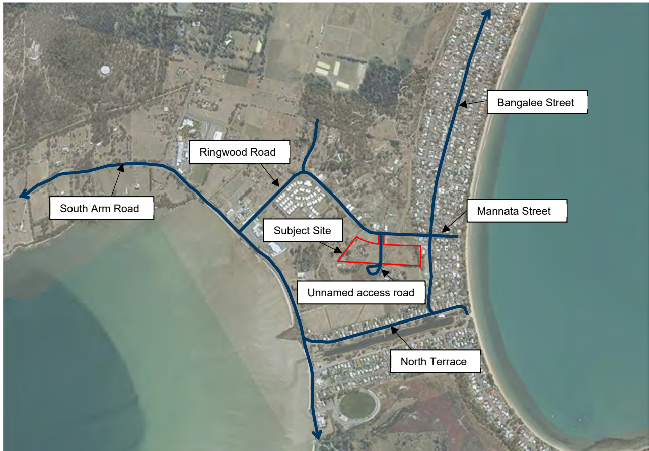
Figure 2.1 Site location and key road network in Lauderdale, Tasmania Base imagery obtained from TheLIST, State of Tasmania, accessed December 2021
