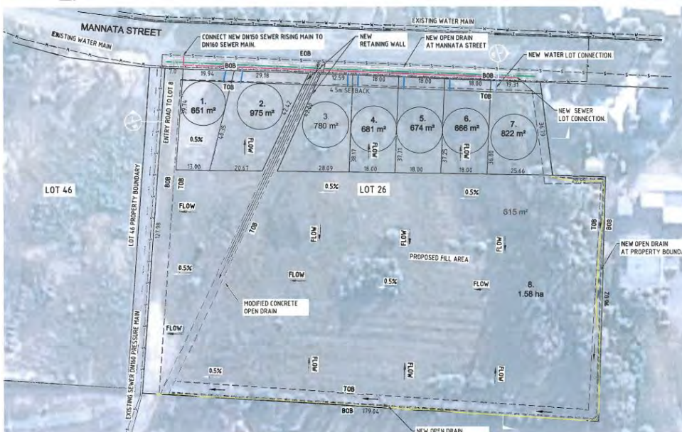
Figure 2 Approved subdivision plan for 7 lots on Mannata Street and approved fill area
