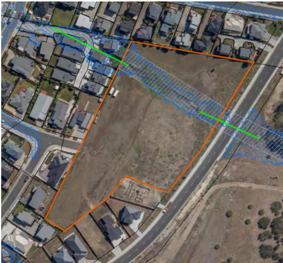
Figure 1 Development site – showing the waterway and coastal protection area, the flood code overlays and the existing 900mm culverts. LISTMap.
